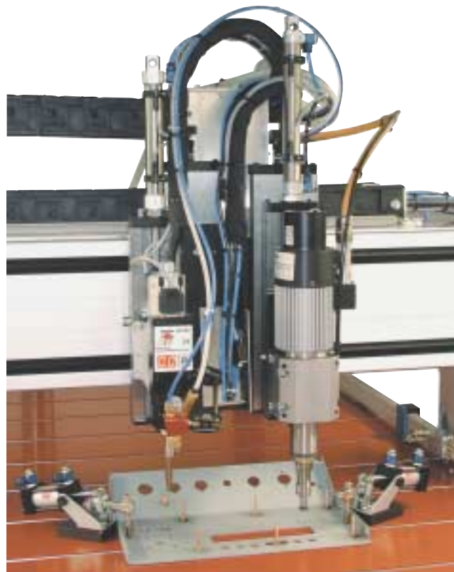
SK-5AP welding head with digital display for precisely measuring the lift and plunging distances combined with a milling/drilling head
